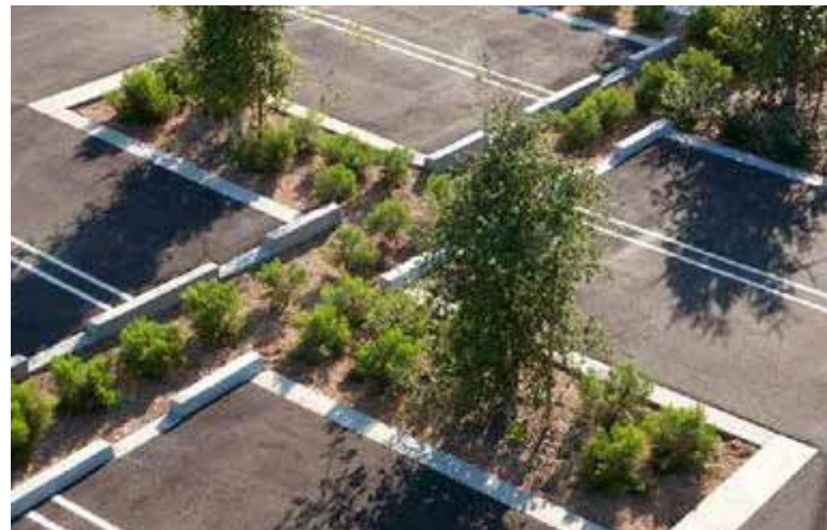
The above images represent ways of using landscape in parking lots to screen parking as well as to filter stormwater and provide a lush verdant pedestrian experience from car to garden entry.
